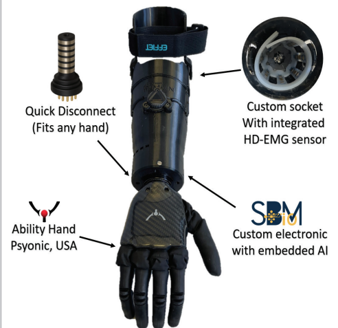
A representation of Félix's myoelectric prosthetic arm. The custom-made socket integrates an electrode array for HD-EMG sensing, a microcontroller for real-time signal processing, and batteries for power. The system can send commands to finger motors of most commercial prosthetic hands.
