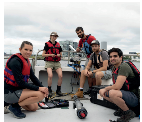
Dariia, Ruby, Rustam, Mat and Edmundo prepare to deploy the ecoCTD (conductivity, temperature and depth instrument) with a dye sensor during OAE field trials
